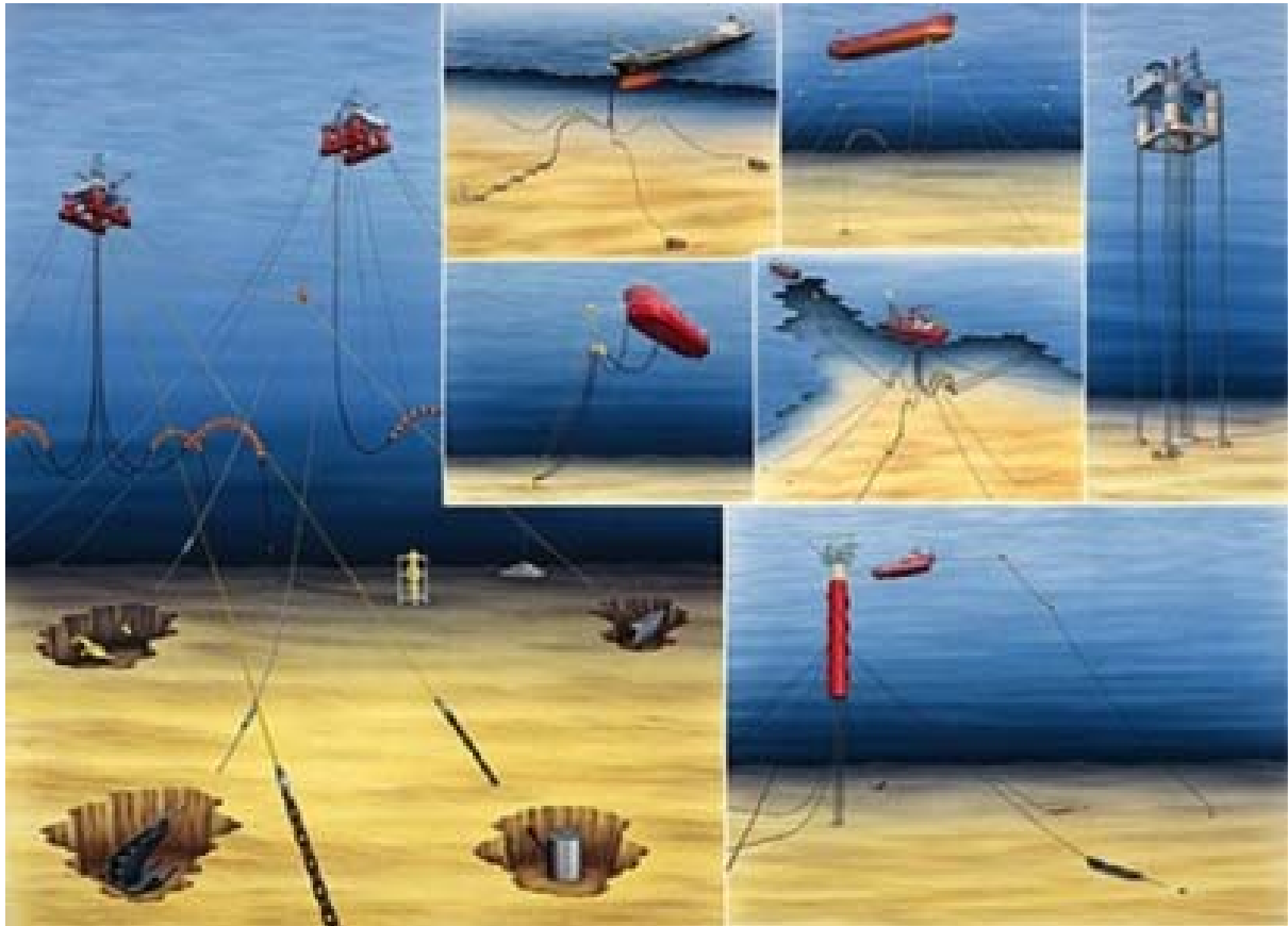
Figure 1. Offshore Mooring Systems
